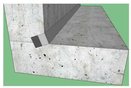
the bottom or from one end until the other on flat surfaces. Using the 2.5 cm margin trowel pack the mixture firmly into the chase. Using a stiff bristled brush wipe the surface area gently insuring a slightly rough surface. Mix only what can be placed in 15 minutes.
