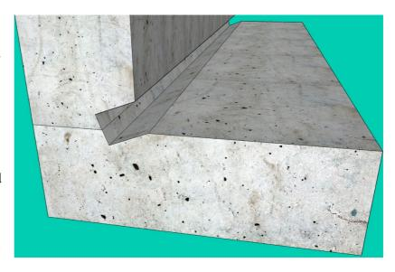
allow 3.5 cm consistently, chip or chisel or route the concrete on both sides of the steel to the appropriate depth and clear the area over the steel to whatever depth is allow by the placement of the steel.
